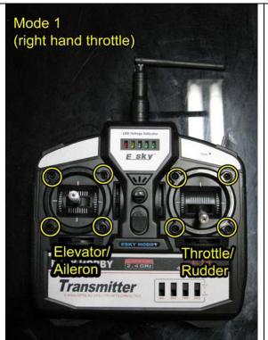
Remove the 8 screws on the front
