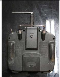
Remove the 6 screws on the back
